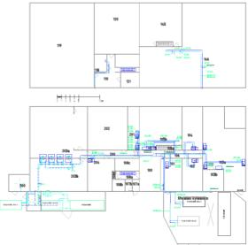
ENACO continued to complement the system's refrigeration pumps with frequency control and replacing valves in fan air coolers. After these rebuilds, several cooling coils could be switched off and instead be stand-by as N+1 backup.
